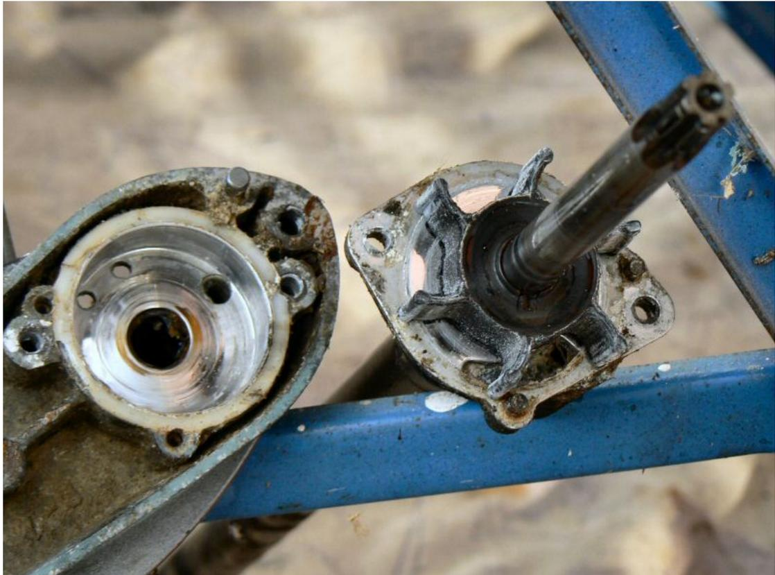
Once separated, the impeller can be slid off the drive shaft. Do not lose the drive pin which is a loose fit into the shaft.
