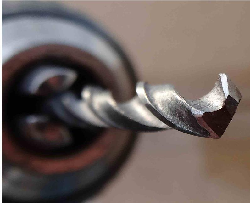
Drill a couple of test holes in the old window to check that the drill bit is producing a clean hole on both sides.
