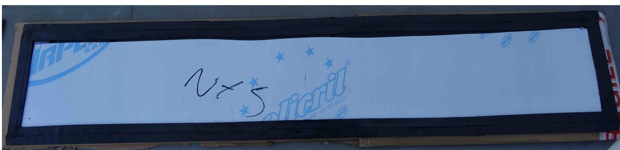
Push a couple of machine screws into the top corners of the window and offer up to the cabin sides.
