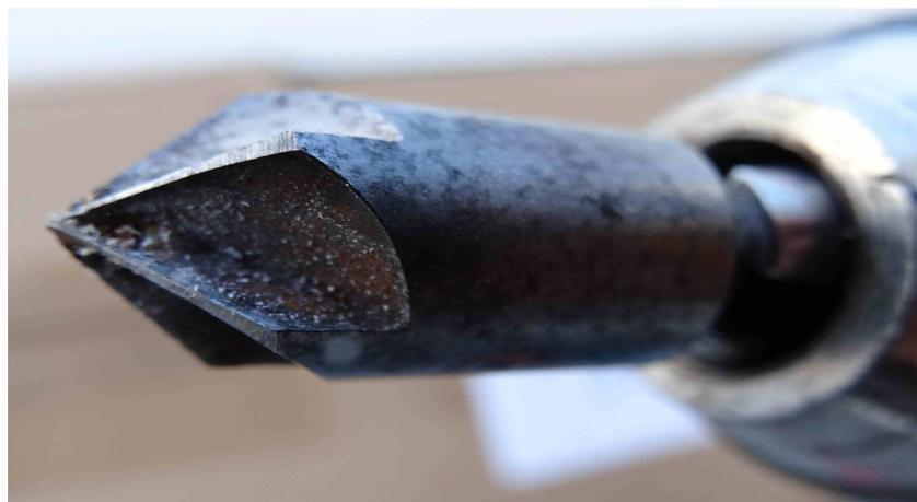
The cabin sides were prepared by countersinking each screw hole. The idea being that the mastic would be compressed into the countersink forcing it around the thread of the screw and, hopefully, ensuring a waterproof seal.
